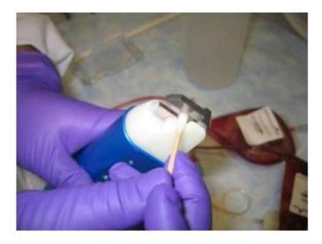
4. Always clean the tubing or freezing bag channels with alcohol before sealing. Moisture or contamination can cause leaks after sealing. Even thin films of contamination or moisture that cannot be seen can cause sealing issues. After cleaning with alcohol, wipe with a dry wipe to remove all moisture.
